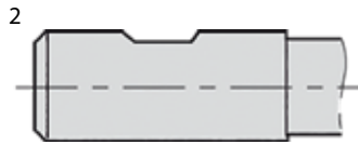
DIN 1835 B/DIN 6535 HB up to \varnothing 20 mm
